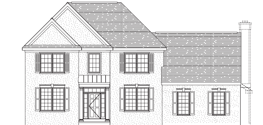
ELEVATION C: Stucco Facade with Front Gables, & Hip Roof Shown with Optional Copper Tone Pent Roof and Chimney
