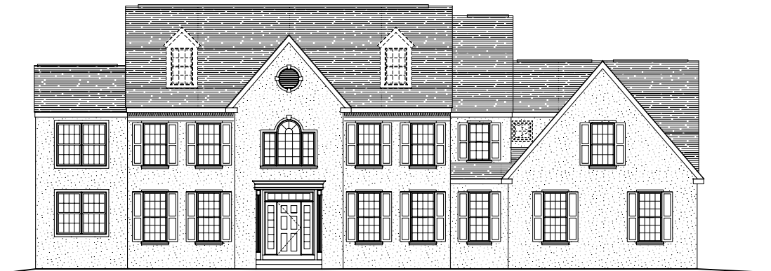
ELEVATION C: Stucco Facade With Center Gable Shown With Optional Dormers & Window at Cricket
