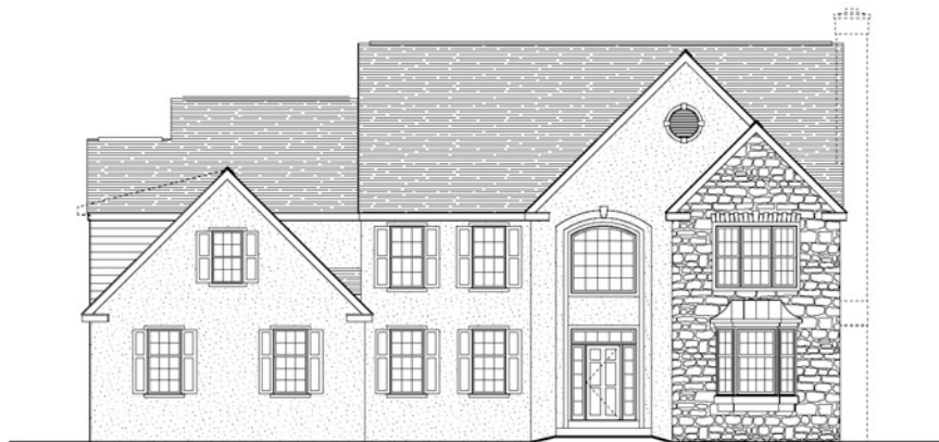
ELEVATION B: Stucco, Vinyl Siding & Stone Facade Shown with Optional Bay Window, Copper Tone Roof & Chimney
