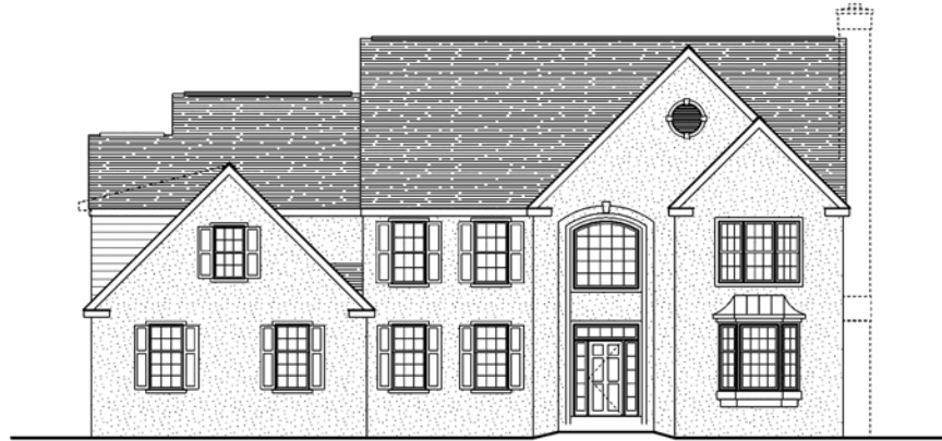
ELEVATION A: Standard Stucco & Vinyl Siding Facade Shown with Optional Bay Window & Chimney
