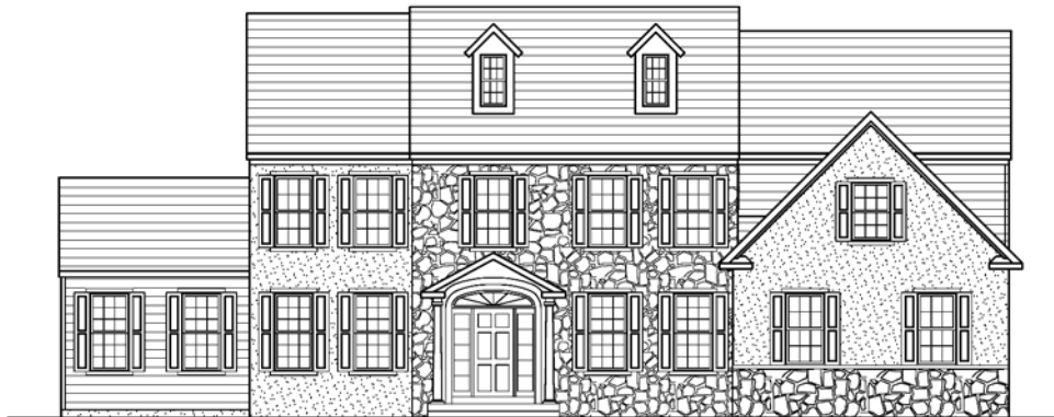
ELEVATION C: Stucco, Vinyl Siding & Stone Facade with Knee Wall Shown With Optional Sunroom, Dormers, & Elliptical Front Pent Roof
